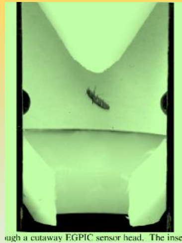
Figure 1. A cutaway EGPIC sensor head. The insect is visible inside the probe.
